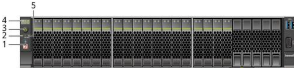
图 5-8: 8x2.5 SAS/SATA+12x2.5 NVMe 硬盘配置前面板指示灯和按钮
